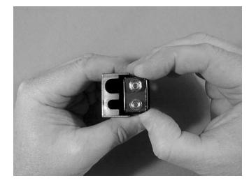
Slide the battery holder into its receptacle in the bottom of the keypad base. It will snap into position.
