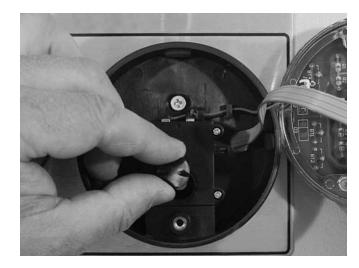
When the disc is positioned correctly, moderate pressure will cause it to snap into place.
