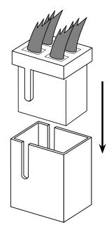
Insert the white power connector into the matching white receptacle on the keypad circuit board. Like the lock cable connector, it will only insert fully when it is oriented correctly.
