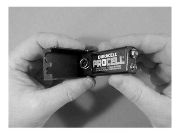
Note that the top of the battery holder is shaped to allow the battery to install only in the correct orientation.
