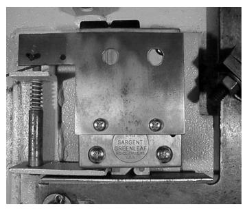
The lock cannot function properly if it binds against the safe's boltwork. It is sensitive to bolt side pressure.
