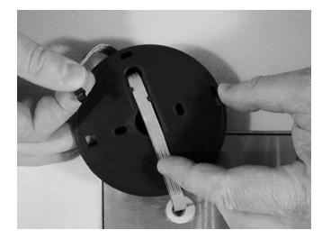
Move the base toward the safe door, gently pulling on the cable to take up any slack. Pull all excess cable through to the front of the keypad base, and make sure it stays in the recessed channel in the back of the base.
