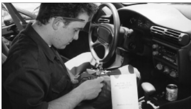
7. Using Blackhawk's progression chart, we can produce a key quickly. Even when all cuts appear as 2/3's, no more than six blanks are needed to produce a working key.
