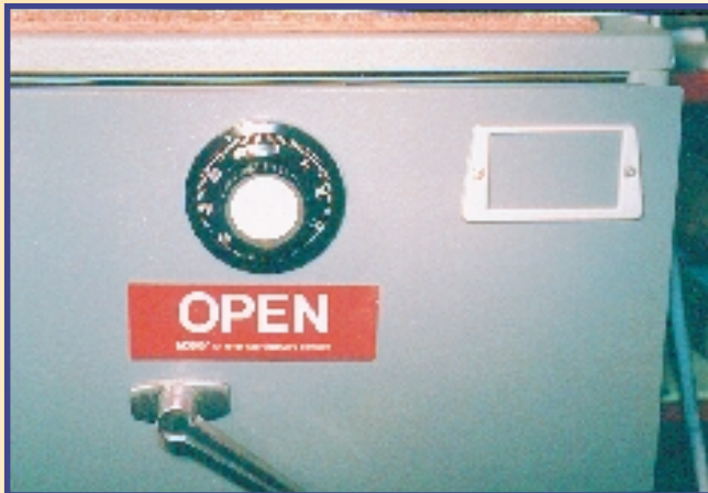
1. Mosler GSA two drawer file cabinet with Ilco (Precision) combination lock in open position and opening handle in down position.
