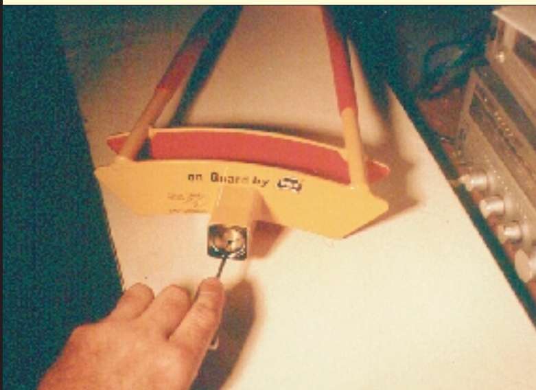
6. A channel found in the lock housing is for the spring operated plunger.
