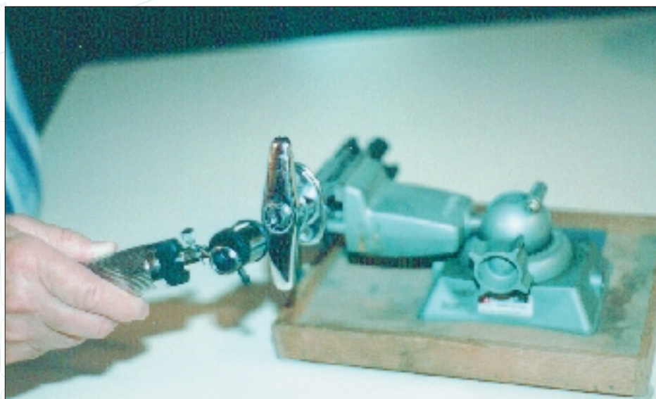
2. Using an otoscope with pin attachment, each wafer tumbler in the lock can be read.
