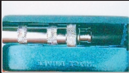
4. An impact driver made fast work of the rusted screws holding the filler plates in place.
