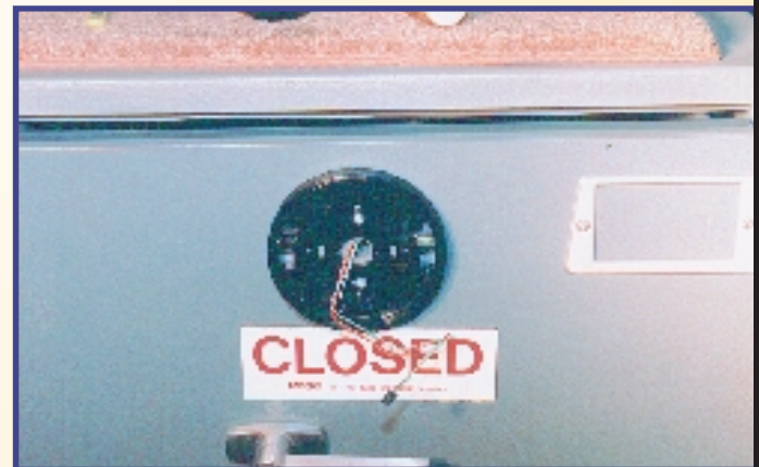
4. The electronic keypad mounting ring with 1/4" connector and cable. Top of ring has no spring clip connector.
