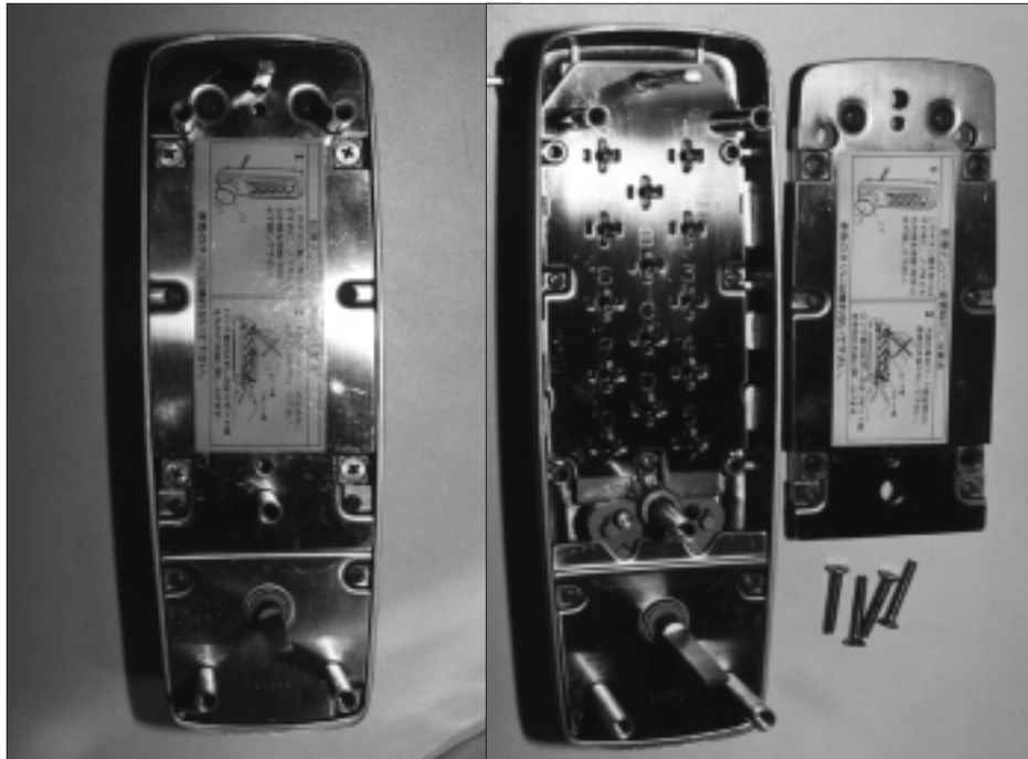
6. Remove the four flat head screws and the backplate.
