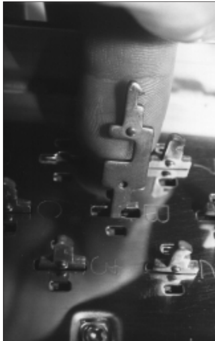
11. Tumblers with gray side up represents the combination.
