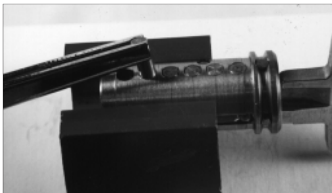
9. Load the conventional pins.
