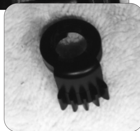
9. The glove box lock is made of plastic and is extremely fragile, and must be removed for lock disassembly.
