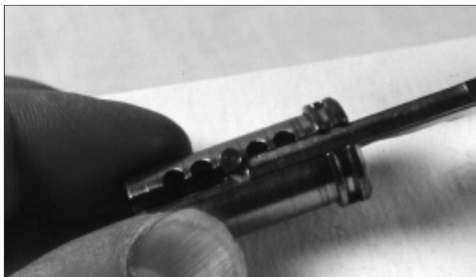
7. Loading the side pins.
