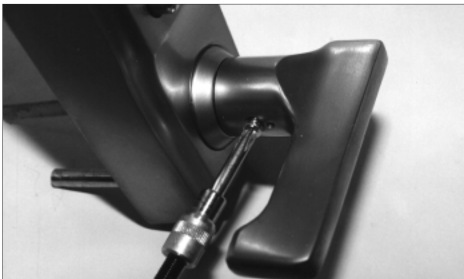
5. Remove the lever screw and lever.
