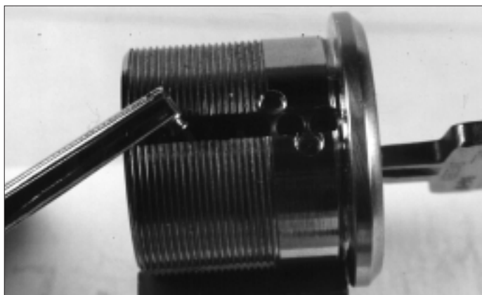
10. When loading from the top, load the drivers with the spool down.
