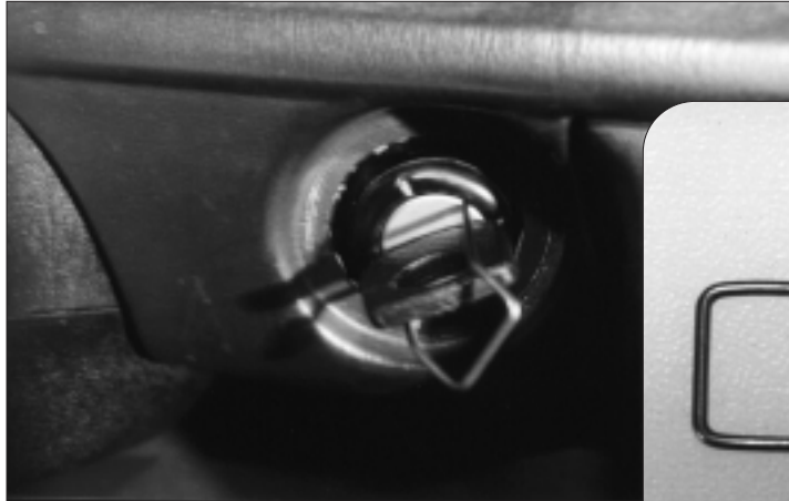
1. After turning the key to the first accessory position, insert this U-shaped wire into the two holes of the lock facecap.
