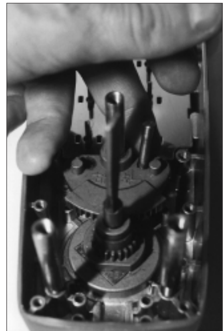
9. Switch the drive pin from one side of the cam to the other and the turn the spindle to finish the handing change.
