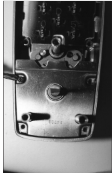
7. Remove the spindle mechanism backplate.
