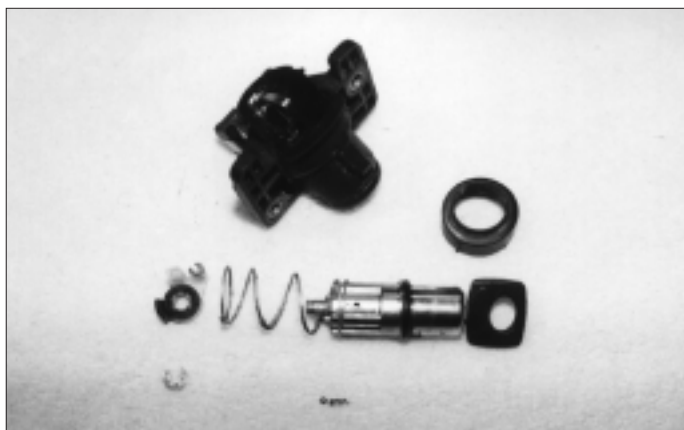
8. The disassembled trunk lock.
