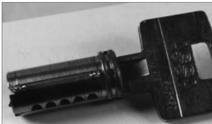
8. Load the sidebar springs and the side bar.
