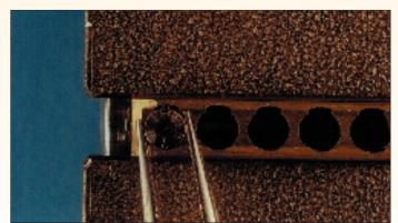
4. Drop the pin into the top of the chamber making sure the locator tab of the tumbler aligns with the locator slot of the pin chamber.
