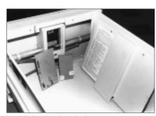
9. Slide the back drawer cover up and remove the two pieces of hard plate.
