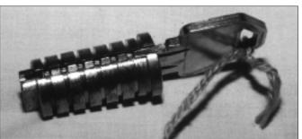
6. The grooves in the plug and the notches at the bottom of the key's blade are necessary to allow the interlocking tumblers to operate.
