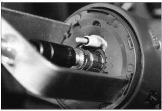
4. Removing the steering wheel lock plate.
