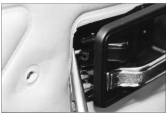
10. Remove the inside release/lock assembly.
