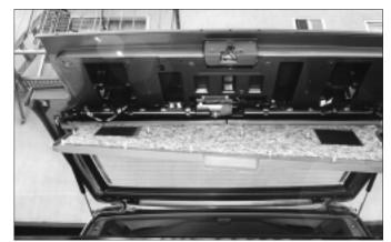
14. To remove the trunk lock the inside rear gate panel must be removed.
