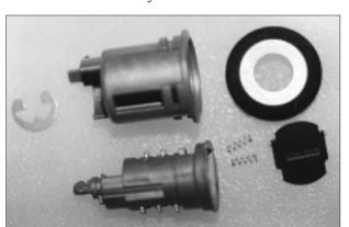
12. The disassembled door lock.
