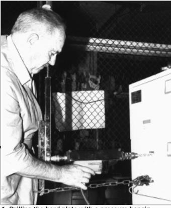
1. Drilling the hard plate with a pressure bar rig.
