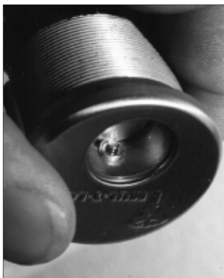
10. Load the combined pins into the shell making sure that the end of the inner pin projects into the plug area.
