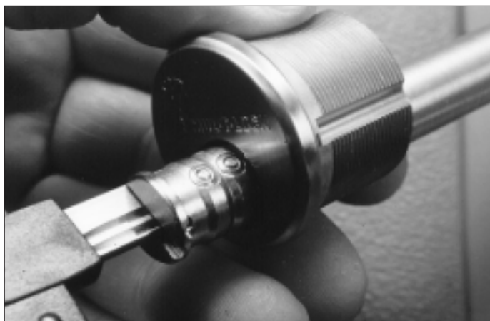
13. Insert the plug into the cylinder shell.
