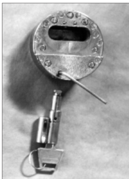
4. Removing the lock cylinder and lock shaft from the lock body.
