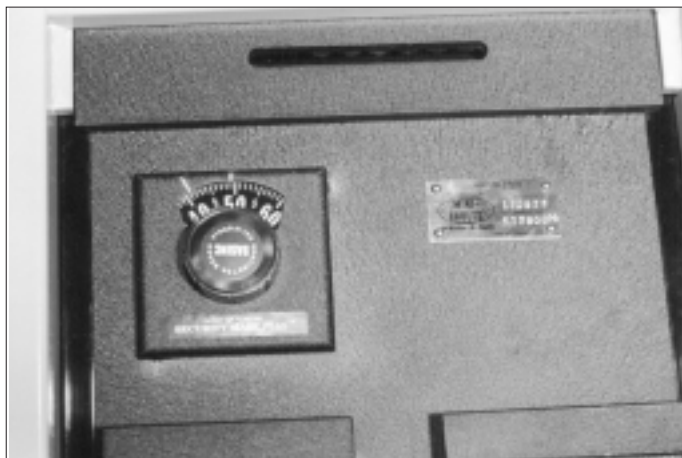
3. View of Mini-Safe with money drop slot installed. The slot has an anti-fish plate on the back.
