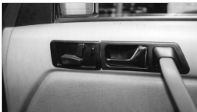
2. Remove the trim around the inside release and electric seat controls.
