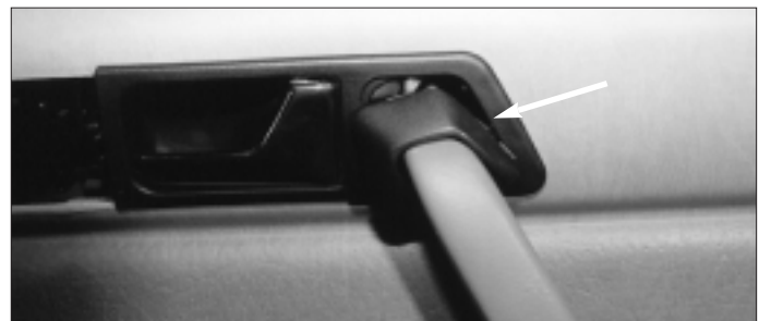
6. Remove the black plastic trim piece that goes around the arm rest/handle, it unsnaps with a little gentle pry from a small screwdriver. Behind the trim piece is a 10mm bolt that must be removed.
