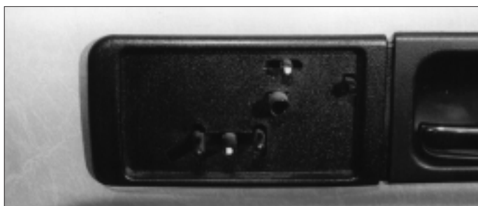
3. The three seat control buttons are removed by gently snapping them off. Below the second largest button is a small black plastic ring that must be gently removed.
