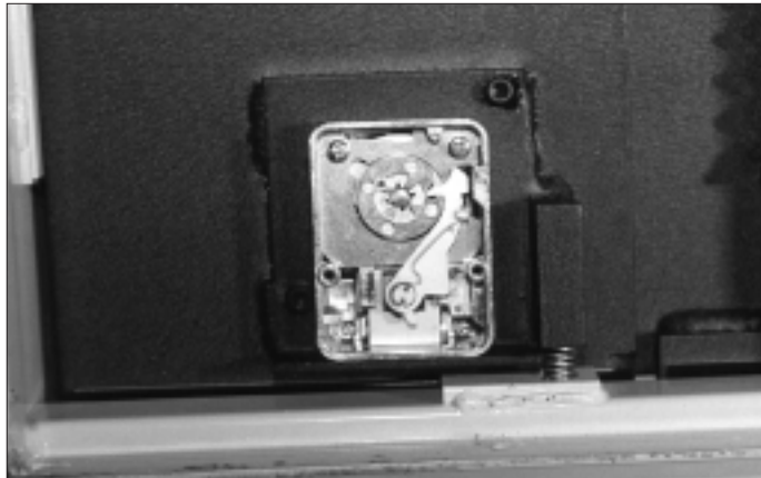
7. Back cover removed releases the spring loaded relock plunger which fires into a reinforced cut out in the door edge.
