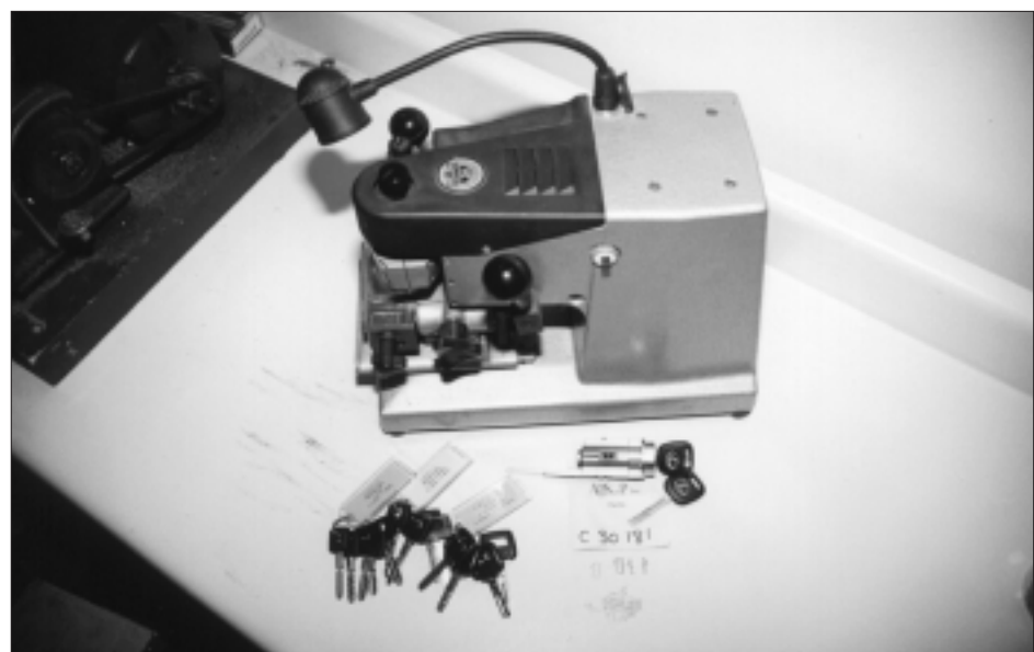
1. A few of the items needed for High Security Auto Service include a high security key cutting machine, depth keys, and replacement locks and service kits.
