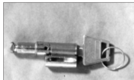
5. Remove the roll pin that holds the shaft to the lock cylinder.
