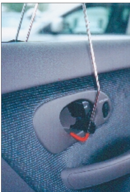
6. As a last resort, pull out on the active release lever and the car will open.
