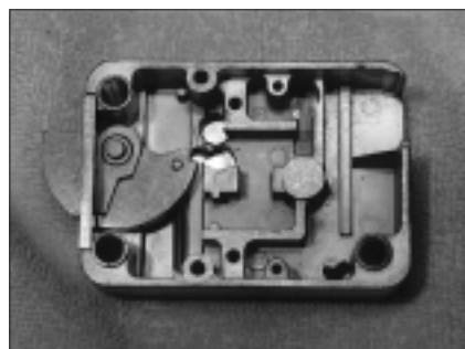
9. Inside of drilled swingbolt lock before I discovered the correct measurement of 1-1/4" toward bolt and 1/4" toward the solenoid.
