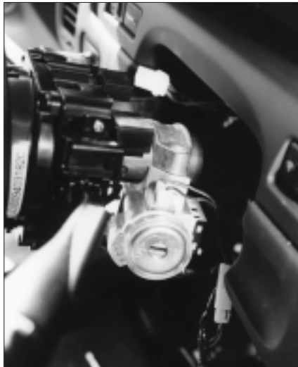
4. The ignition lock with shroud removed.
