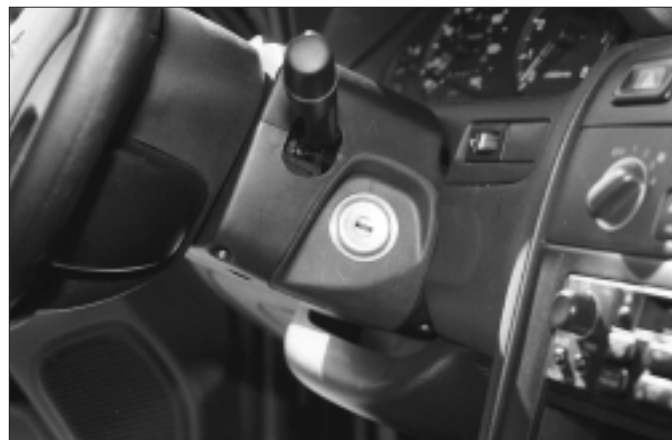
3. A view of the ignition and the two piece clam shell column shroud.
