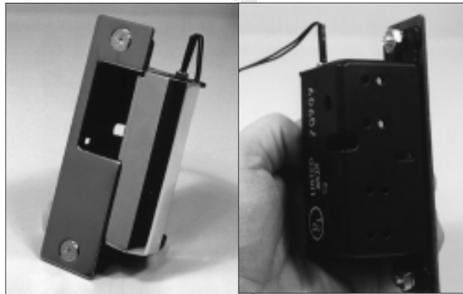
1. This HES 1003K electric strike has the solenoid tucked away in its lip, making it virtually impervious to mortar dust problems. The small chassis area makes it ideal for mortar filled steel frame installations.
