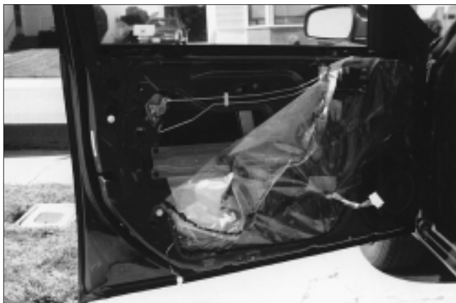
9. With the door panel removed the lock and lock linkage can be seen.
