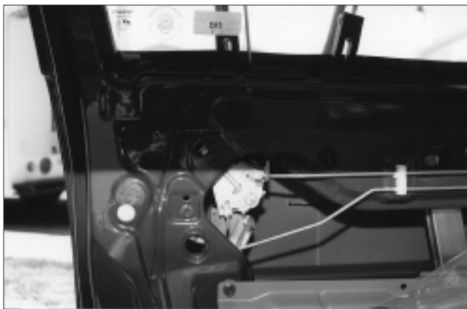
2. The horizontal linkage must be grasped up near the bell crank and moved forward.
