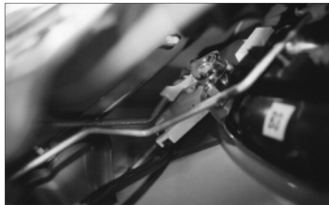
10. In order to get to the lock cylinder, the bell crank, linkage shield, door support and window track must be removed or loosened.
