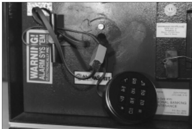
7. Setup for opening safe, keypad attached to double female connector which is now attached to the safe wire.
