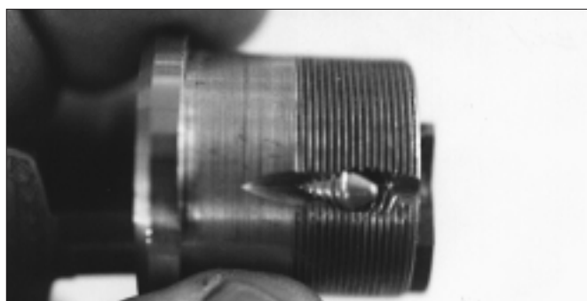
4. This set screw helps prevent the lock from being forcibly unscrewed from the lock case.
