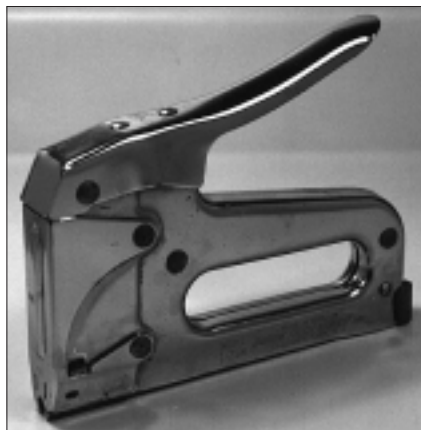
1. Stapling is one of the most common wire fastening methods used by the electronic locksmith.
