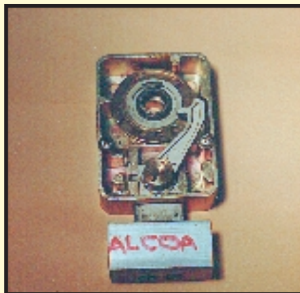
5. Front of the lock with attached ALCOA aluminum blocker block attached. The block measures 1"x1"x2".
