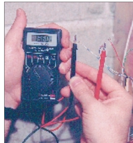
5. Use the voltmeter to determine which lines are Telco lines and which are premises phone lines. The 41.7 volt reading indicates the Telco line; the 136 millivolt (a fraction of a volt) reading indicates the premises phone line.
