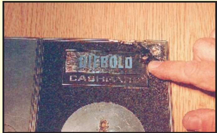
2. The hidden corner screws that hold the escutcheon to the door.
