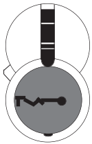
1. Load pins with plug turned.
